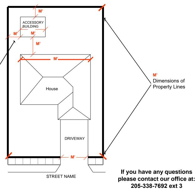
Site Plan may be hand drawn using a ruler, but must be drawn to scale.
